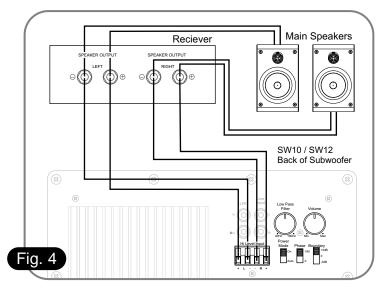
With all signal connections complete, it is now time to apply AC power. Plug the power chord into the power inlet in the back of the subwoofer, plug the other end into into the wall outlet and switch the subwoofers power to the ON position.
